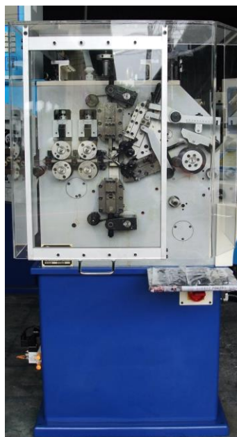
Safety wiring, interlock cover for CE standard
